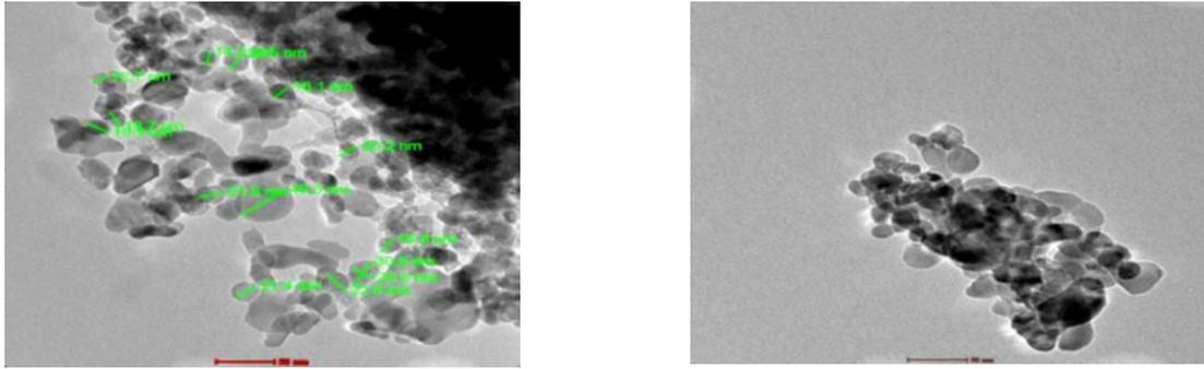
Fig. 1. Scanning electron microscope images of zinc oxide nanoparticles (ZnO-NPs).
