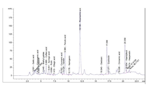
Fig. 2. HPLC Chromatograms of standard metabolites showing signal from diode array detector at wavelength 280 nm. Peak: Rosmarenic acid, Ferulic acid, Coffeic acid.
