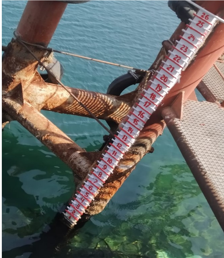
Fig. 1. Tamasa is used to measure the water level at the Sea Hydrometeorological Station of the “Neft dashlari” in the Caspian Sea.
