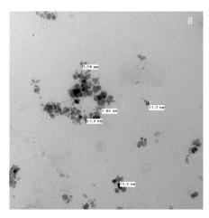
Fig .1b. TEM of Capsulated 3 % thyme oil with nano-chitosan
