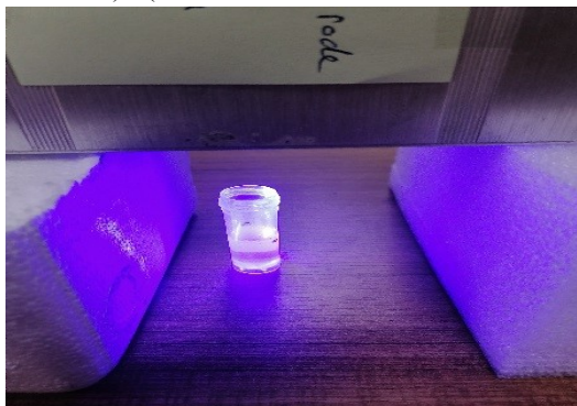
Fig. 2. Illustration of the use of laser radiation on the crude petroleum ether extract produced from leaves of Populus spp.
