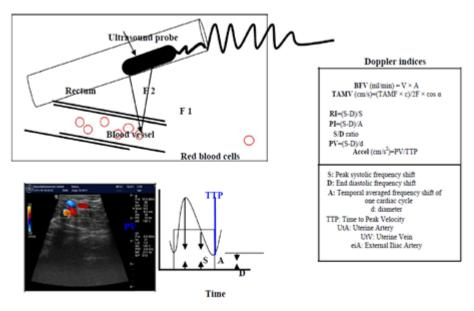
Fig. 8. Semi-quantitative evaluation of blood flow by determination of the resistance to blood flow using the Doppler indices RI and PI. D, end diastolic frequency shift; M, minimum frequency shift; S, systolic frequency shift; TAMF, time averaged maximum frequency shift.
